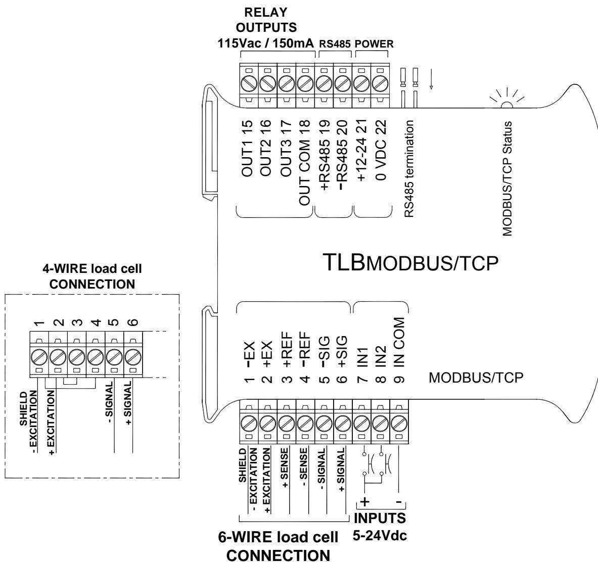
**3 outputs:** settable setpoints or remote output management via protocol.
