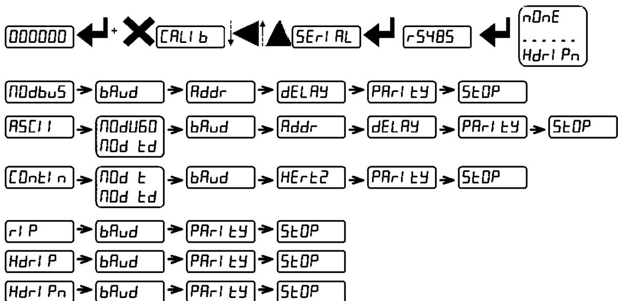
According to the chosen protocol only the necessary settings will be displayed in sequence (see diagram here above).
