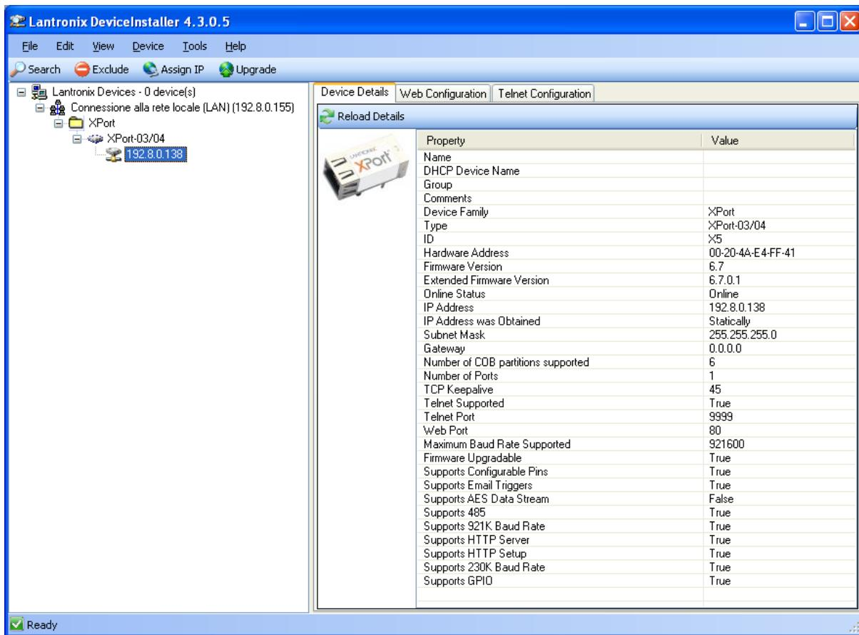
In the left pane, select the device found. Press the "Assign IP".
